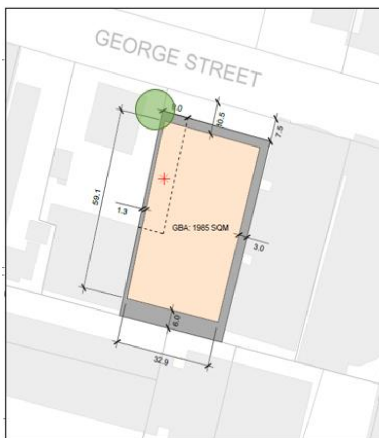
Figure 3: Option B as preferred by the applicant. The podium is in grey and tower in beige. The rectangular area identified by the red asterisk reflects a 9m setback from the western boundary for the lower levels of the podium only.
